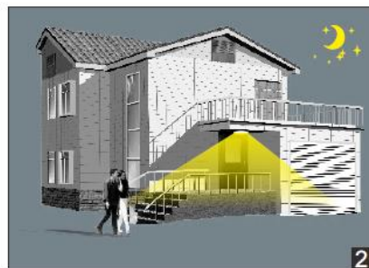
2 With insufficient ambient light, the sensor switches on the lamp when motion is detected.
